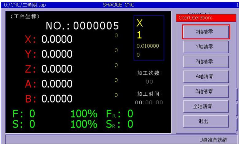
X axis single axis clear Y axis single axis clear Z axis single axis clear A axis single axis clear B axis single axis clear
