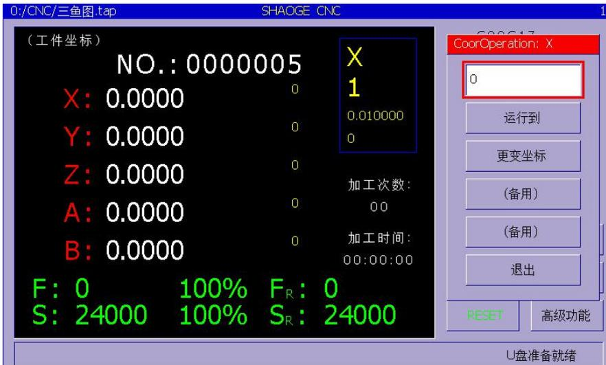
The "run to" axis will directly run in the specified coordinates.
