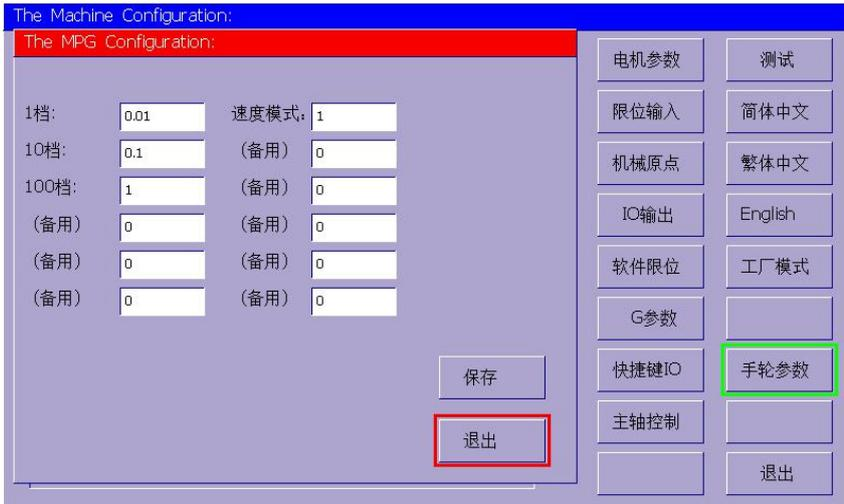
1st file: the length of each step of x1 corresponding to handwheel, generally 0.01mm
