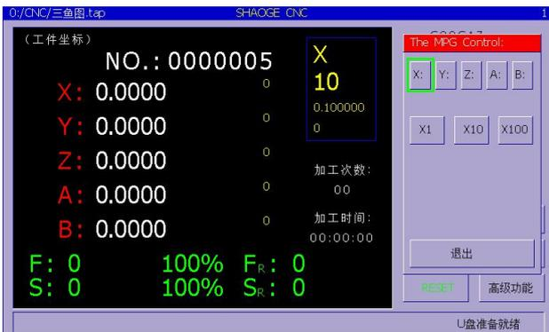
After calling the panel hand wheel operation, the blue basket handwheel parameter items in the screen will be displayed.
