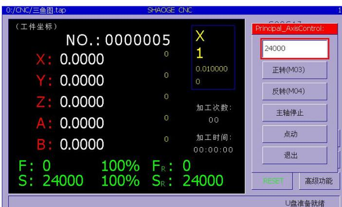
The input basket can be filled with the number of revolutions. The highest value of this parameter can be set in the host settings.
