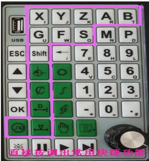
The panel shortcut key X Y Z A B is "direct coordinate operation"
