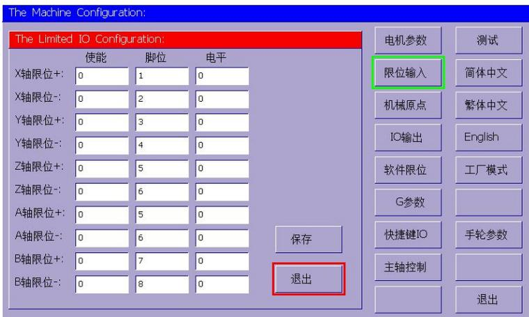
The limit input is generally based on the maximum value of the stroke of the machine table. Once touched, it will cause an emergency stop and no deceleration. Protection does not exceed the mechanical stroke type.
