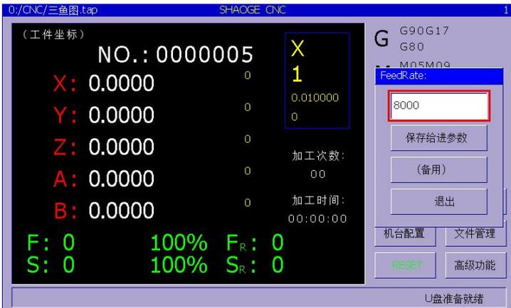
The value in the display basket is the manual feed speed of the navigation key and does not affect the highest speed of the handwheel.
