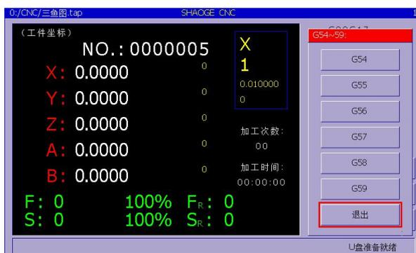
When G\* is selected, the coordinate system of the seat can be selected and it needs to cooperate with the mechanical coordinates.
