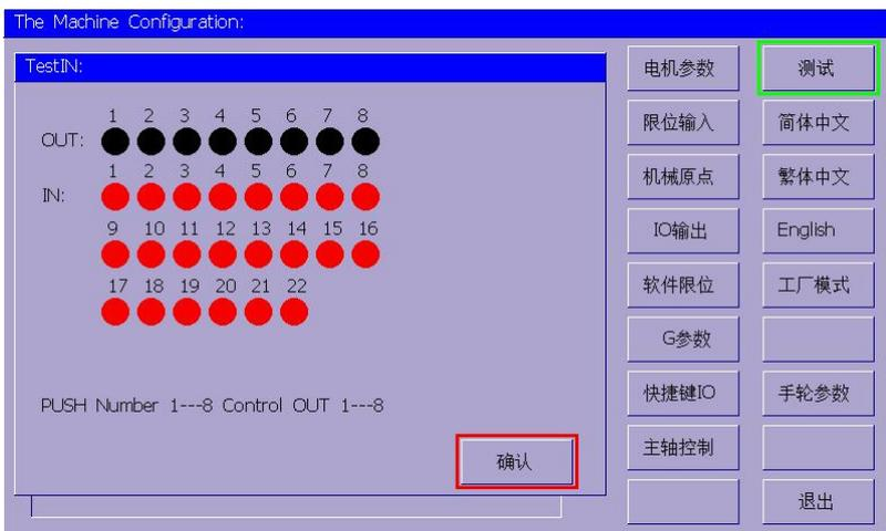
Press 1-8 on the panel to control the output port number 1-8. Check if the input is normal.
